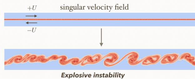
The mixing layer reaches a finite size in a finite time, even when the initial perturbation is sent to zero
