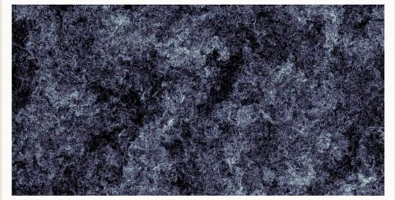
Local energy dissipation in a slice of a three-dimensional homogeneous turbulent flow at  $Re_\lambda \approx 730$ .
