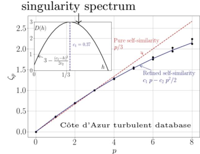
**Multi-fractals:** Range of scaling exponents  $h \in (h_{\min}, h_{\max})$
